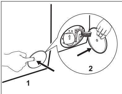
2. Place a suitable bowl below the drain pump access to collect the water that flows out.
