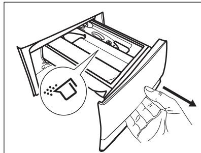
2. Press the lever down to remove the dispenser.
