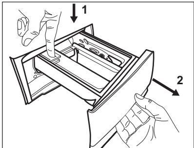
2. Remove the top part of the additive compartment to aid cleaning. Make sure that all detergent residue is removed from the upper and lower part of the recess. Use a small brush to clean the recess.
