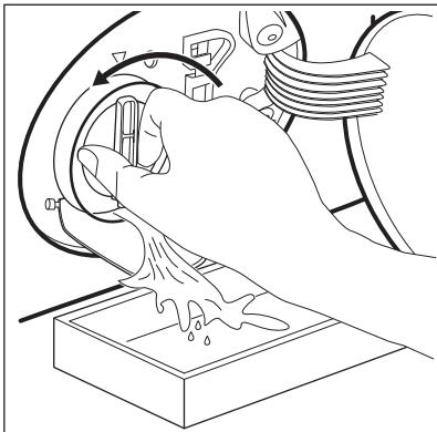
5. When the bowl is full of water, turn the filter back and empty the container.
