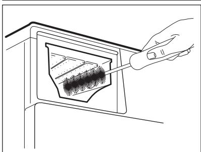
3. Flush the detergent drawer out under running warm water to remove any traces of accumulated detergent. After cleaning, replace the top part in its position.
