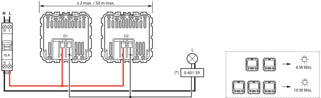
(\*) For some electronic loads, the installation of a compensator Cat. No. 0 401 39 is required.
