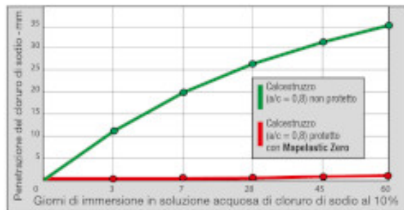
Fig.3: Effect of Mapelastic Zero on the penetration of sodium chloride into a porous concrete
