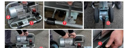
The housing can be bolted to the ground (7) or secured with a strap (11) and suitable load attachment accessories via the fastening lug (8) to a fixed object (e.g., a tree). You can also used the latching bolts (6) to secure the housing on the RUNPOTEC trolley (10) on the rail. The trolley itself can be bolted down, attached directly to a trailer hitch (12) or fastened to a fixed object with a strap fed through the fastening lug (11).
