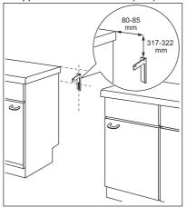
2. You can find the hole on the left side at the back of the appliance. Lift the front of the appliance and put it in the middle of the space between the cupboards. If the space between the bench cupboards is larger than the width of the appliance, you must adjust the side measurement to centre the appliance.
