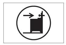
Install the anti-tilt protection 317 -322 mm down from the top surface of the appliance and 80 - 85 mm from the side of the appliance into the circular hole on a bracket. Screw it into the solid material or use applicable reinforcement (wall).
