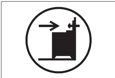
1. Install the anti-tilt protection 317 - 322 mm down from the top surface of the appliance and 80 - 85 mm from the side of the appliance into the circular hole on a bracket. Screw it into the solid material or use applicable reinforcement (wall).
