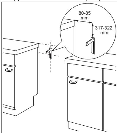
2. You can find the hole on the left side at the back of the appliance. Lift the front of the appliance and put it in the middle of the space between the cupboards. If the space between the bench cupboards is larger than the width of the appliance, you must adjust the side measurement to centre the appliance.
