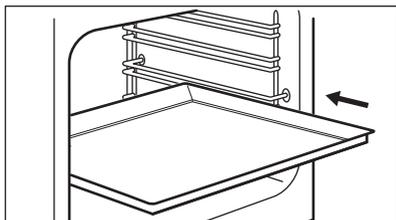
Push the tray or deep pan between the guide bars of the shelf support. Make sure it does not touch the back wall of the oven.
