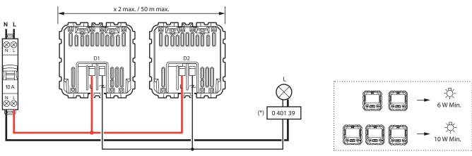
(\*) For some electronc loads, the installation of a compensator Cat. No. 0 401 39 is required.
