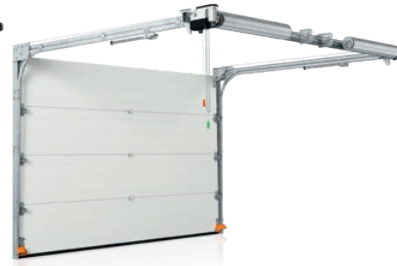
LH – low tracks – torsion springs at the back
